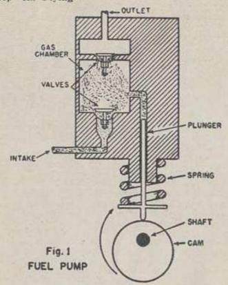
Fuel injection pumps are usually operated by a cam and spring. The cam moves the plunger during the delivery stroke and the spring returns it during the suction stroke. The cam is coupled with the engine crankshaft by means of gears or chains. Fuel is drawn into the gas chamber during the suction stroke and forced out during the delivery stroke.
